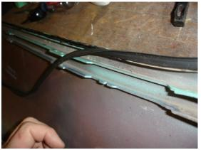
I used some clamps for the front cladding. There is a slot so you'll know it has to be installed in just the right location. The extra beading in the front wraps around so you don't need to trim it.
