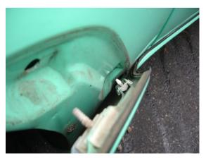
Now move to the front cladding. Remove the single bolt from the bottom of the cladding using the 10mm socket. Then remove the plastic access plate from the front wheelhouse by removing the two Phillips screws. Turning the wheel makes access easier. Once removed, use the 10mm short socket to remove the bolt that is holding the front cladding in place. There is another placement bracket here. Put it aside along with the bolt.
