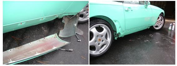
I choose to replace my stone guards. These come off with the application of heat. Then you'll need to get the adhesive off. Once everything is clean I used my polishing wheel and clean the side of the body. Then, pull the stone guards off of their backing and cover the sticky part with a soapy-water solution. Then apply to the body and position to the right location. Use a plastic edge to squeeze the soapy water solution out to the sides.
