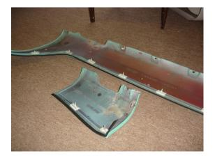
Start with the front cladding. Install the piece by pressing in the 1 clip and then follow by attaching the nut to the bolt. Make sure your positioning bracket is in the place you took it off and holding the extra beading piece that is wrapping around the corner down tight. Hold the cladding tight to the body as you tighten down the nut. Not too tight, it's a plastic nut. Now install the one bolt on the bottom.
