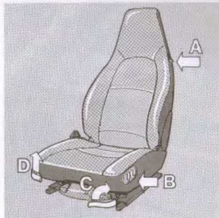
A Backrest release B Height adjustment C Fore-and-aft adjustment D Backrest adjustment
