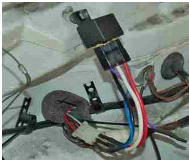
THE RELAY WILL NEED TO BE WIRED ACCORDING TO THE WIRING DIAGRAM ON THE NEXT PAGE, OR YOU CAN BUY ONE FROM [WWW.968ENGINEERING.COM](http://WWW.968ENGINEERING.COM) ALREADY PIGTAILED AND TERMINATED WITH THE PINS THAT ENGAGE THE KEY SWITCH CONNECTOR.
