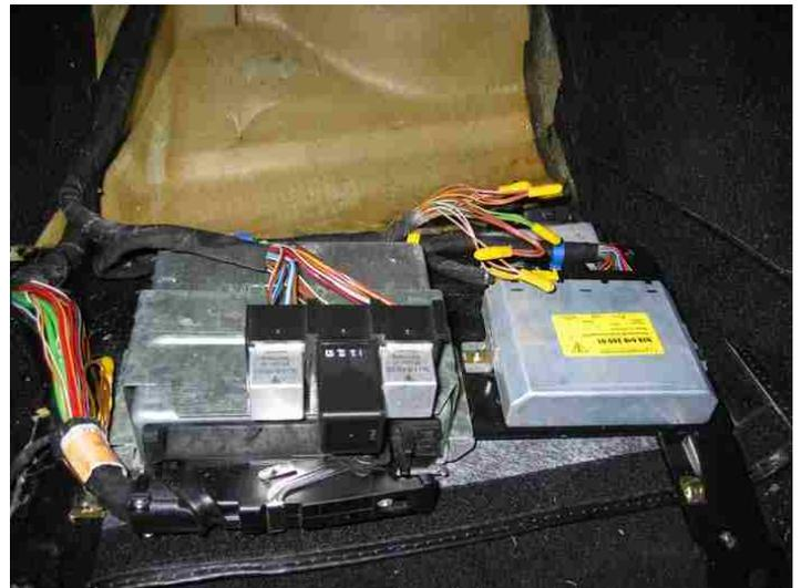
2. NEAR THE ALARM COMPUTER, THERE IS A LOOSE WIRE BUNDLE WRAPPED UP IN BLACK INSULATION. UNWRAP THAT BUNDLE TO EXPOSE SEVERAL WIRES TERMINATED WITH YELLOW CAPS. FOR THE DOOR LOCK FUNCTIONS YOU WILL NEED TO UNCAP THE FOLLOWING WIRES:
