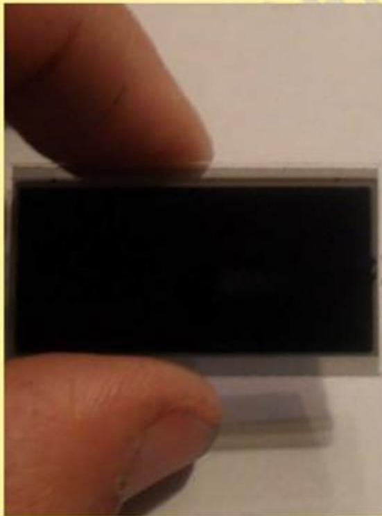
The housing has a "notch" to allow the LCD to seat fully forward, If the LCD doesn't want to sit flat, this is probably your problem.
