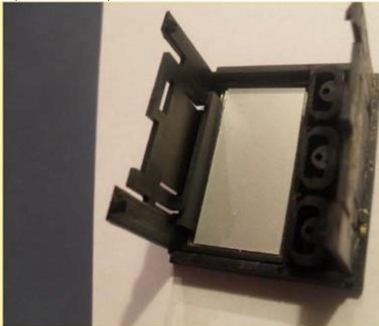
Next put the plastic deflector in place and insert the other connector block in the gap. Do make sure you get the paper back in as it does serve a purpose in light transmission .
