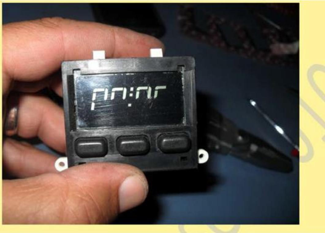
Lower section of LCD is not making contact on this one. Sometimes the plastic strip behind the LCD gets in the way. See bottom of page 4 in the center. This piece can easily interfere with the connectors. You can leave it out as once the unit is installed back in the face plate of the dash, you will not see the edges and it will not make much difference when installed.
