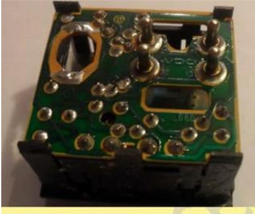
You will want to apply power to check the function of the LCD, you can also install the LED for the clock at this stage. Please note that the LED can only work with current flowing one direction, so if it will not light twist it 180 degrees. Be gentle, it is possible to break the board (ask me how I know).
