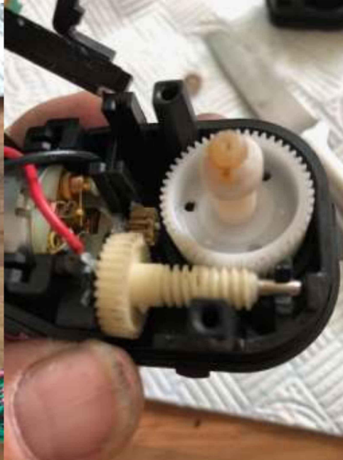
A good helping of white silicone grease is a good thing to fill this up with, I kept it clean so I could do the photos
