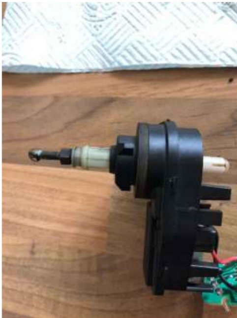
A good helping of white silicone grease is a good thing to fill this up with, I kept it clean so I could do the photos
