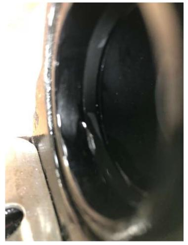
Now for the pistons, this is a one shot deal normally, once in they are a pain to get back out without blanking off all the holes and compressed air, so I fit the dust boots / seal first then polish the piston with a decent microfiber cloth,
