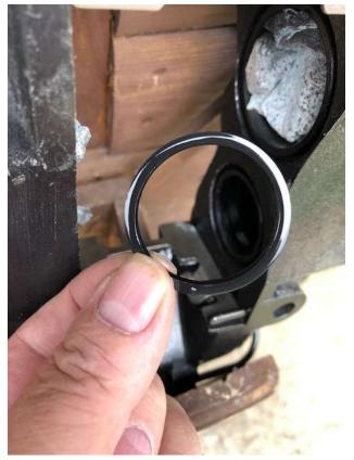
A 36mm Seal fished out its conditioner bath, the fitting is in good old Haynes fashion, just steer the seal into the groove with your finger tip and start to push all the way round and it will just pop in
