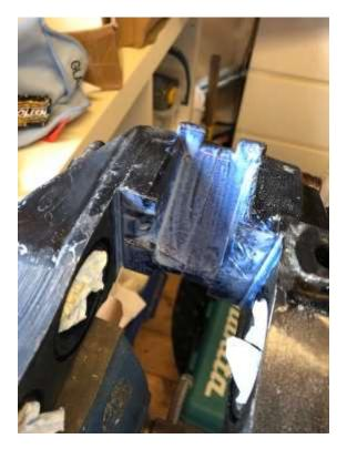
I have removed the bleed nipples and I tried to get a close up picture of the crap down the bleed hole, more corrosion due to infrequent fluid changes, brake fluid is hydroscopic so absorbs water and when its in a tight space possible for years and years , the result is in the picture.
