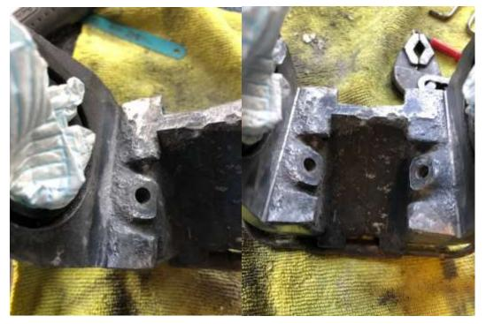
Now reached the point with all the corrosion removed and just bright shiny alloy to see, now we need to protect it, I really don't think some of the tricks used are a good idea, like silicone between the plates and body, one little pocket fills with moisture and away it goes and you can't even see it, anyway I'm going to coat it with a water based corrosion barrier that once dry is as hard as steel.
