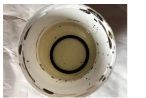
First thing to do when you are ready for this part is the new seals need soaking for at least 24 hours in the Brembo Seal Conditioning fluid, So do this well in advanceNew 36mm Seal having a paddle....
