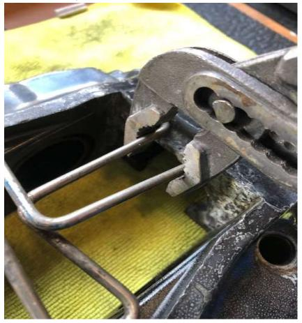
A big squeeze and up and down movement helps free them off, they also required a tap or two with a small hammer to get them out, the holes are full of rubbish, using a pick and brush I get them clean
