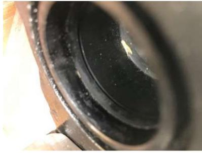
Here is the seal sitting in its groove, when you look closely you can see the seal is sitting at an angle making the the bottom or inside edge higher than the top edge, this provides the fluid seal and also aids piston insertion, the new seals are totally square cut so there is no wrong or right way to fit them, the grooves the seals sit in are machined at an angle
