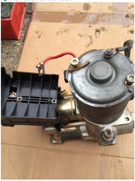
4. Remove the motor from the valve block should be nice and clean inside
