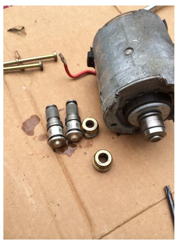
Put these in the 968 pump same method, put the repaired pump back in the car and then bleed the brakes furthest point first NS rear caliper.
